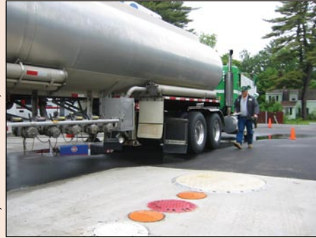
This type of fuel delivery truck most often makes gravity deliveries.
