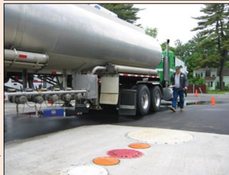
This type of fuel delivery truck most often makes gravity deliveries.
