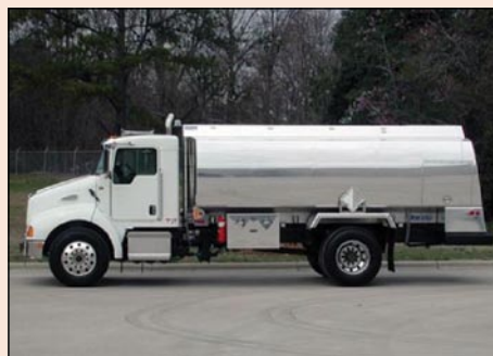
This type of fuel delivery truck most often makes pumped deliveries.
