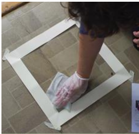
Above: Home lead dust testing involves taking samples of a square foot area of two floor surfaces (shown here) and a windowsill which are analyzed at HETL to see if there is any lead dust present in the samples.
