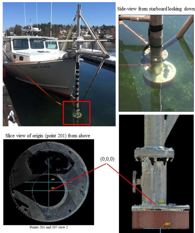
Figure 5 – Amy Gale origin (point 201 in RGB images) for vessel reference frame(s); origin is center point within the base of the pole (center point of base within internally-mounted motion reference unit (MRU) point 201 in images above)
