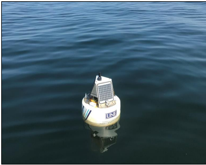
Above: The real-time acoustic receiver deployed in southern Saco Bay by Dr. John Mohan and his research lab.
