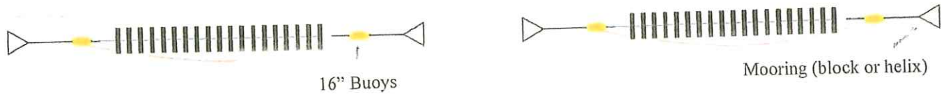
Overhead close-up view of lines showing buoys and mooring
