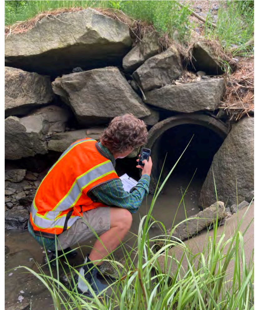
FIGURE 3.6 - Low-tide observations and photo documentation are essential elements of Rapid Site Assessments. Photo by Slade Moore.
