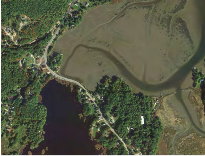
FIGURE 1.6 - This road dams a former tidal inlet of the Kennebec River estuary. Remnants of tide mill dams are in the adjacent mudflat and inlet to the east. Photo source: Google Earth.
