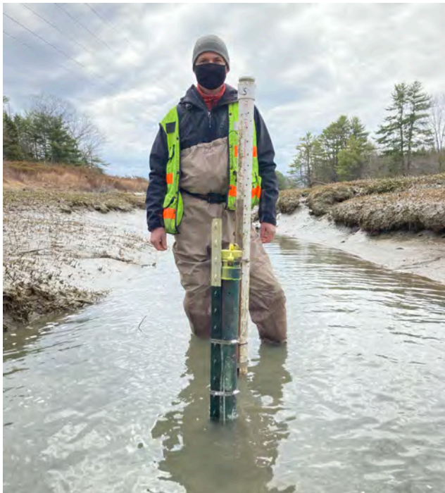
FIGURE 4.2 - Water level monitoring instruments installed in a representative channel reach of a salt marsh. Photo by Slade Moore.
