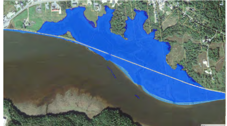
FIGURE 3.4 - Example of simulated present sea-level HAsT inundation extent for existing site configuration (lighter blue) and proposed conditions (darker blue, barely visible at north margin).
