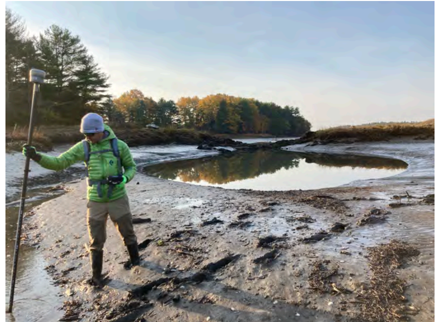
FIGURE 4.1 - Real-time kinematic GPS receivers are one of several tools that are typical of elevation surveys. Photo by Slade Moore.
